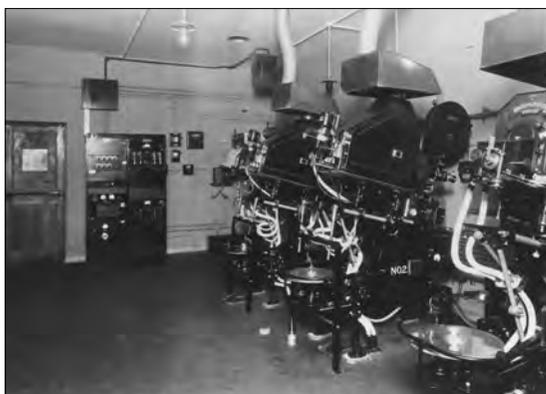
Fig. 4.1 The projection booth of a cinema in Tooting, South London, circa early 1930s. The projectors are equipped both with optical sound-on-film reproducers and turntables (underneath lamphouse) for Vitaphone records. Courtesy of BFI Stills, Posters and Designs.
